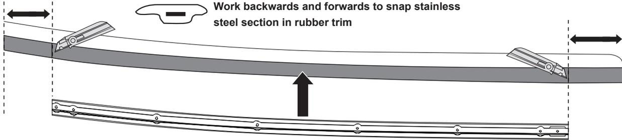
Work backwards and forwards to snap stainless steel section in rubber trim
