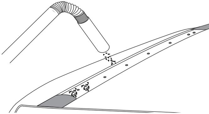
Use a vacuum to remove swarf to eliminate scratching. Wipe clean the installation area of the roof.
