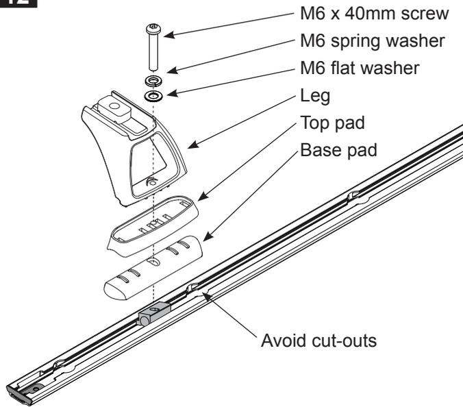
Attach the legs to track using supplied screws and washers. Finger tighten only.
