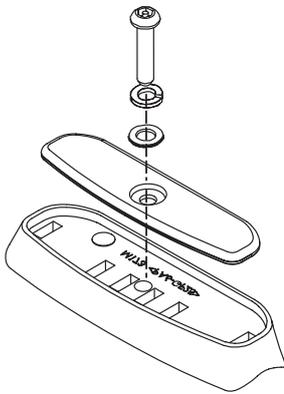
Pad cover plates are provided for when crossbars are removed.
