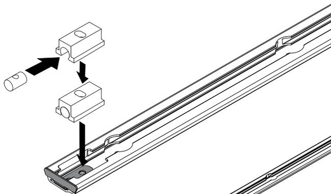
Locate dowel nut into aluminium housing. Slide into track. Slide to approximate position of where you want the cross bars.
