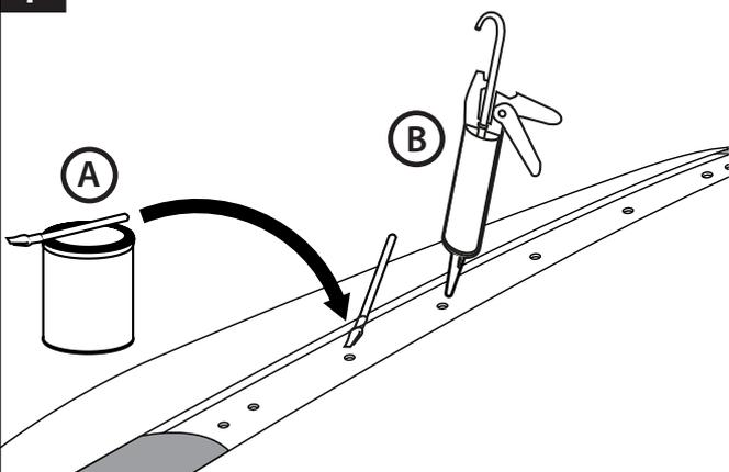
**A.** Apply a liberal amount of cold galvanizing solution to the inside and surrounds of all holes. Allow cold galvanizing solution to dry as per instructions (5-10 mins in hot, dry weather. Longer in cold, wet weather)
