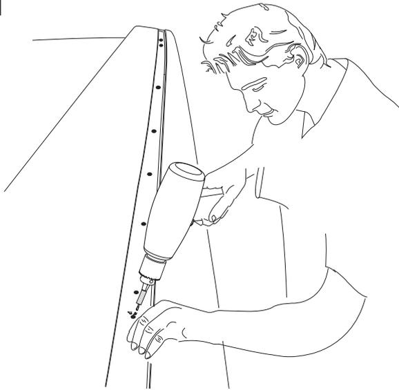
All 8 holes can now be drilled through. A drill stop must be used to prevent drilling through the hood lining on the inside. **Make sure that when drilling you hold the drill perpendicular to the roof angle.** The roof skin is approx. 2-3mm thick.
